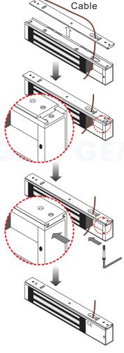
1.Pass the power cable through the mounting plate and the hole of the maglock.
